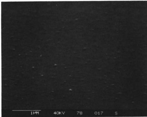
Fig.5: SEM micrograph of a 40 nm thick Y_2O_3 film deposited at 773 K
